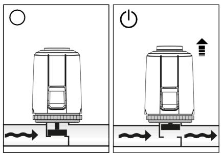
Normally closed (NC): The Function display extracts when the valve opens.
