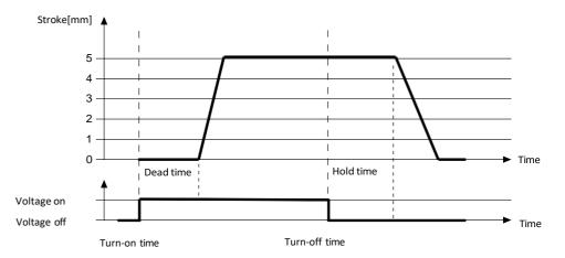
The valve is opened steadily by the plunger motion upon switching on the operating voltage and after expiry of the Dead time. After the operating voltage is cut and after expiry of the Hold time the valve is closed evenly by the closing force of the compression spring. The actuating force of the compression spring is matched to the actuating force of commercially available valves and keeps the NO valves closed when de-energized.
